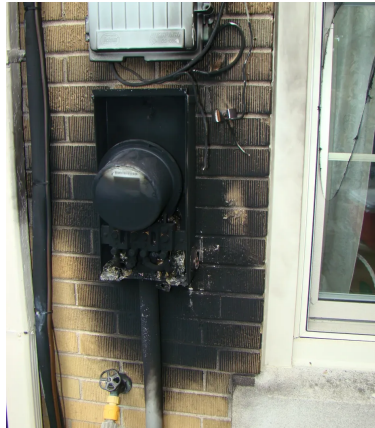
Charred remains of a burnt smart meter
